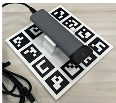
Figure 6. 3D-printed plate with ArUco markers to determine reference object orientation for ablation study.
